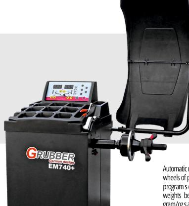
POWER SUPPLY: 230V/50Hz POWER CONSUMPTION: 180W MAX. WHEEL WEIGHT: 65 kg RIM DIAMETER: 10"-24" 1,5"-20" RIM WIDTH: ACCURACY: 1g BALANCING TIME: 8s NOISE LEVEL:  $< 70 \, dB(A)$ 5-50°C WORKING TEMP .: WEIGHT: 60 kg
